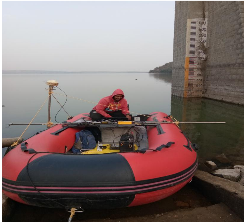
Configuration of SBES Equipment
